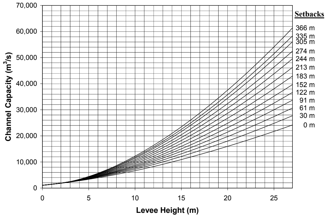
Figure 4.4. Stage-discharge rating curves at 12.5 km from the confluence with Sacramento River (7.75 river mile) for 13 different levee setbacks.
