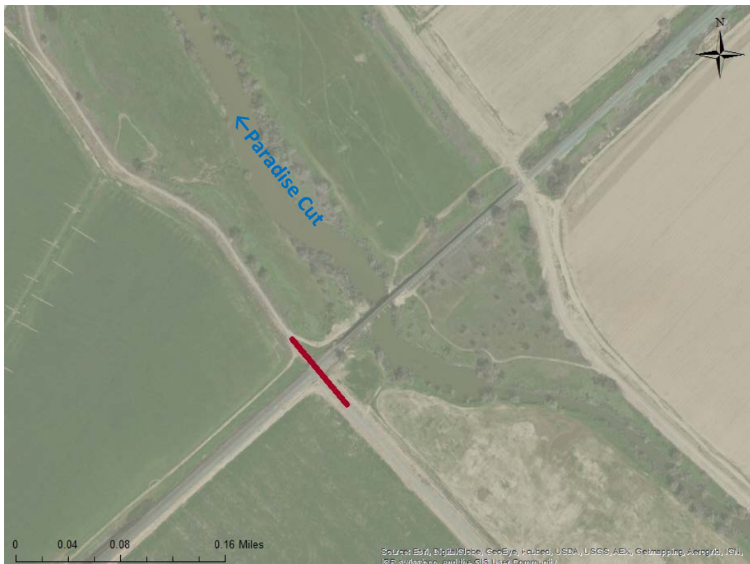
Figure 3-4. Widen UPRR #2 by 160 feet new alignment
