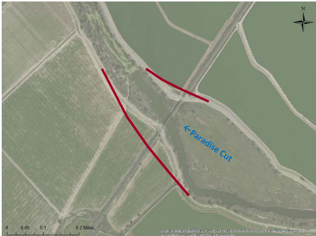
Figure 3-3. Widen UPRR #1 by 400 feet new alignment
