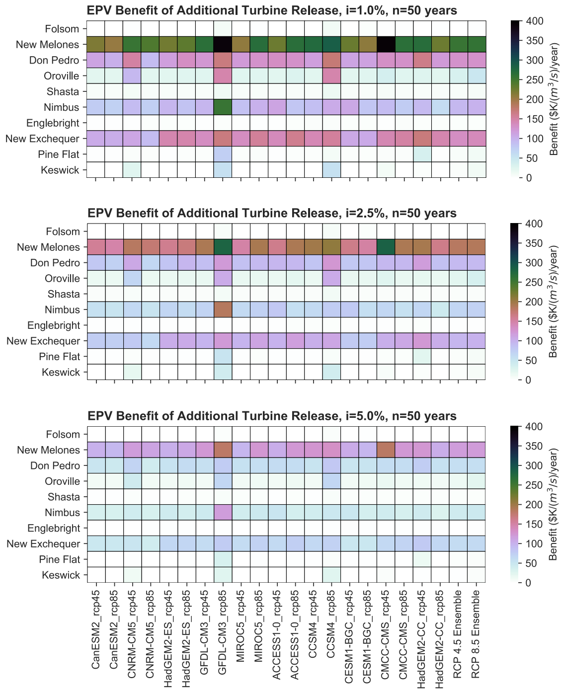
Figure 4.22: Expected present value benefits ( \$/m^3/s/year ) of additional turbine releases with 50 year return for low (1%), medium (2.5%), and high (5%) interest rates
