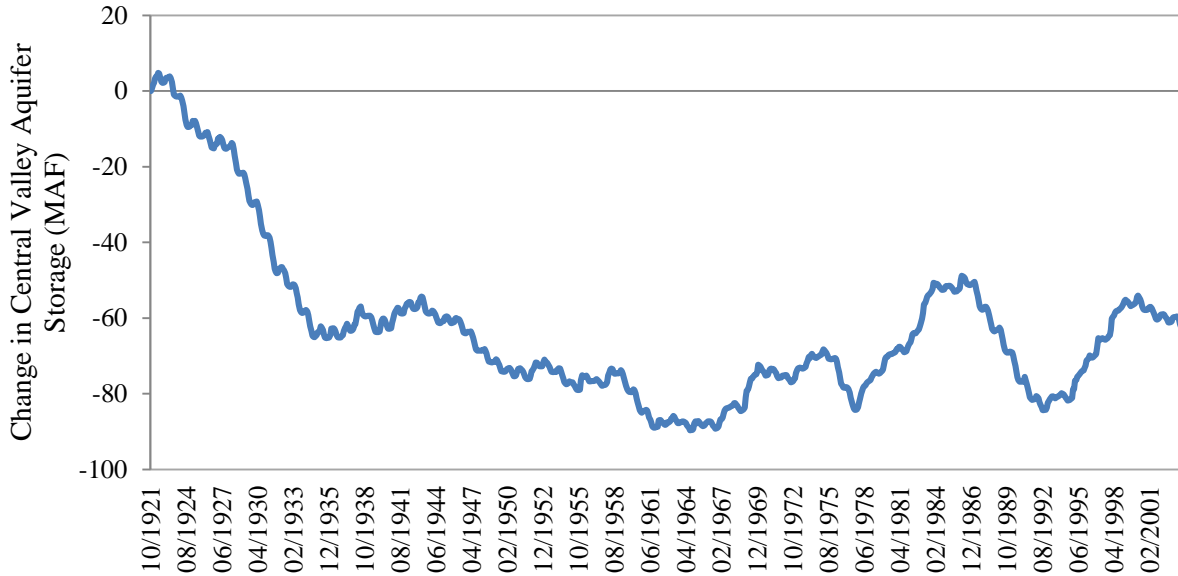
Figure 37. Change in monthly storage in the Central Valley aquifer with unconstrained overdraft over the 82-year period
