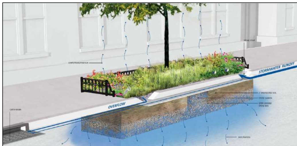
Figure 4: Diagram of a curbside rain garden (Source: Partenio 2020)
