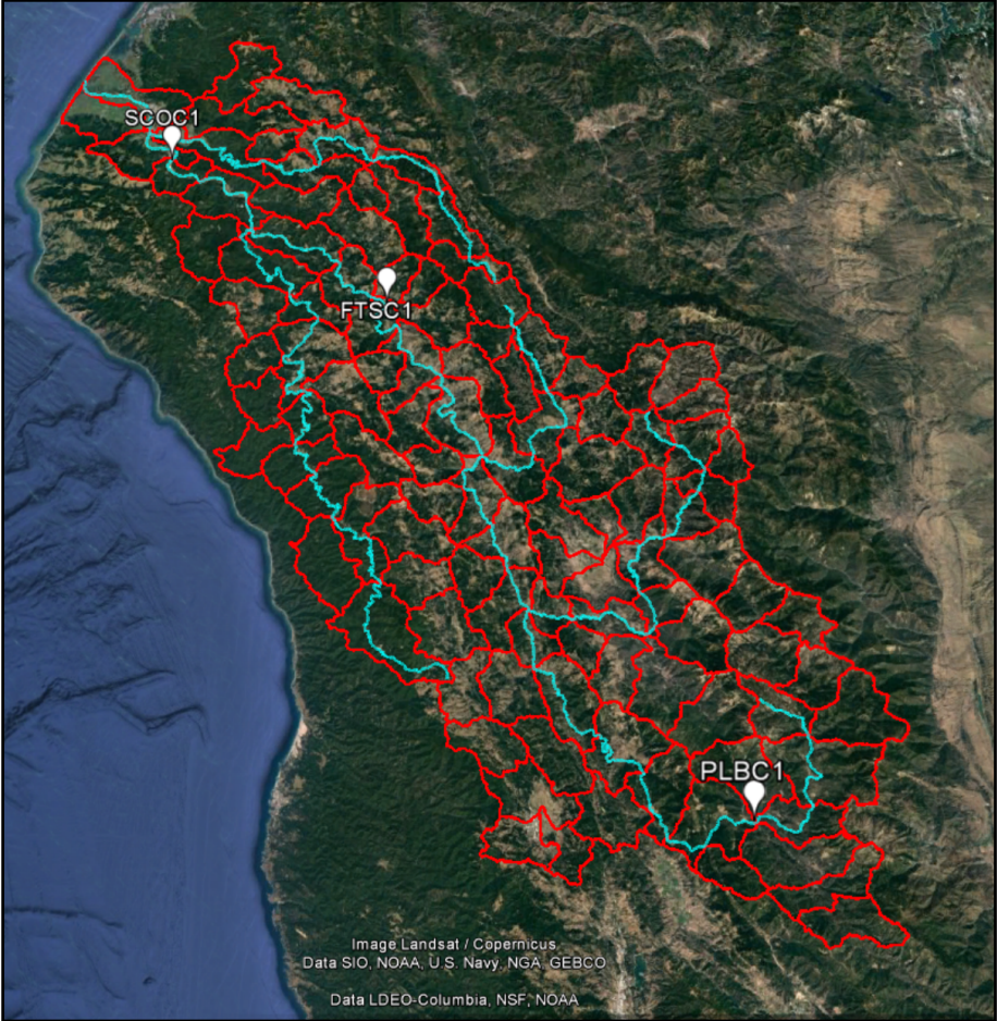
Figure 3: In the Eel River basin, the DWRAT model bases its flow predictions on data from 3 gages: one each from Scotia, Fort Seward, and Lake Pillsbury.
