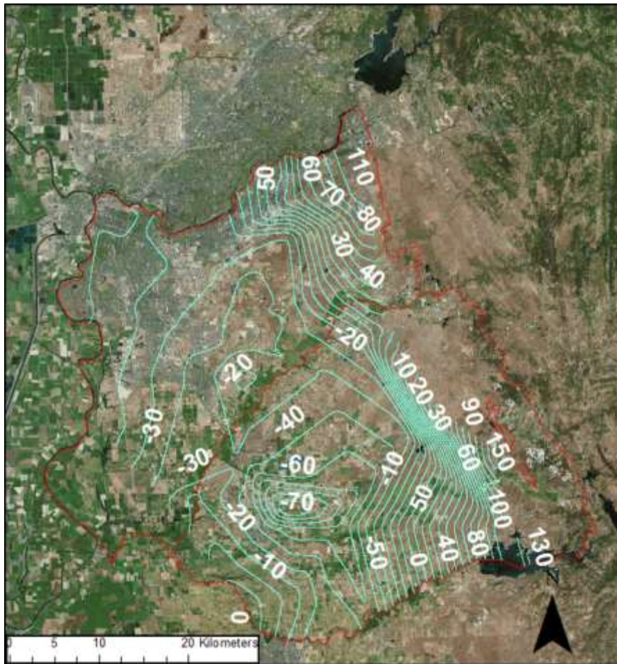
Fig. 48: Groundwater levels in the study area for Fall 2017. Contours are in ft msl. Data source: https://gis.water.ca.gov/app/gicima/ . Land surface elevation ranges from approximately 0 ft msl in the southwest to 400 ft msl in the northeast
