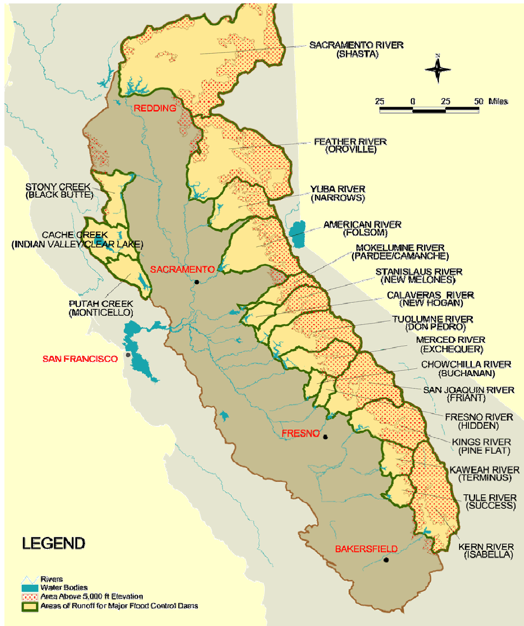
Figure 1. Major watersheds that drain the western slope of the Sierra Nevada into the Sacramento-San Joaquin Valley. The polka-dotted areas indicate elevations above 5000ft, a crude estimate of the rain-snow boundary elevation. If warm temperatures accompany a storm, rain can occur at the highest elevations. Likewise, if temperatures are cold, snow can fall on the valley floor. The Upper Sacramento and Feather rivers are the most northern basins on the map. New Bullards Bar is located within the Yuba River watershed and abuts the southern boundary of the Feather River watershed (Figure taken from Collins and Whitin 2004).
