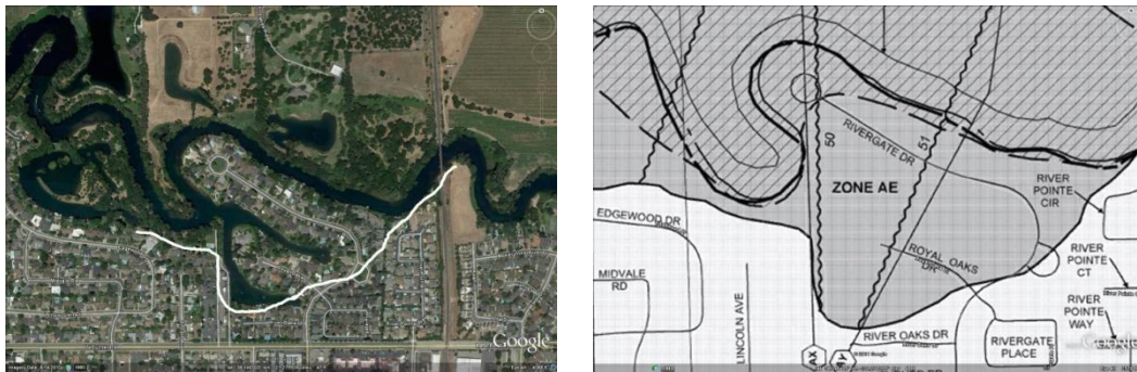
Figure 9. Aerial photo (left) of the Lodi peninsula and the FEMA 100 year floodplain (north of white line). FEMA map (right) indicates different levels of flood risk with shaded areas (100 year) and non-shaded (500 year). Most of Lodi is within the 500 year floodplain.
