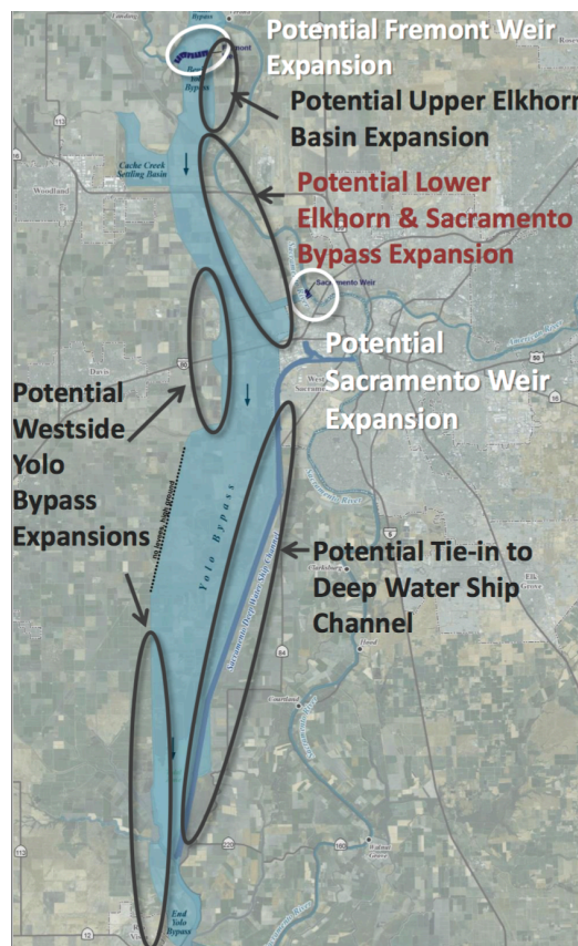
Figure 4.3 Potential flood and ecosystems improvement to the Yolo Bypass system Source: DWR, Yolo Bypass Implementation Status & The Path Forward (May 20, 2016) Update to Central Valley Flood Protection Board
