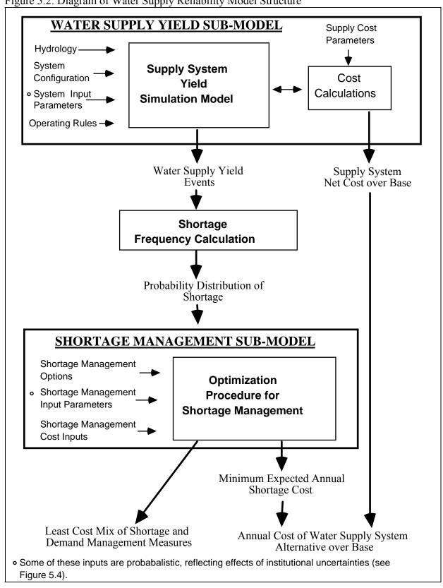
Figure 5.2: Diagram of Water Supply Reliability Model Structure
